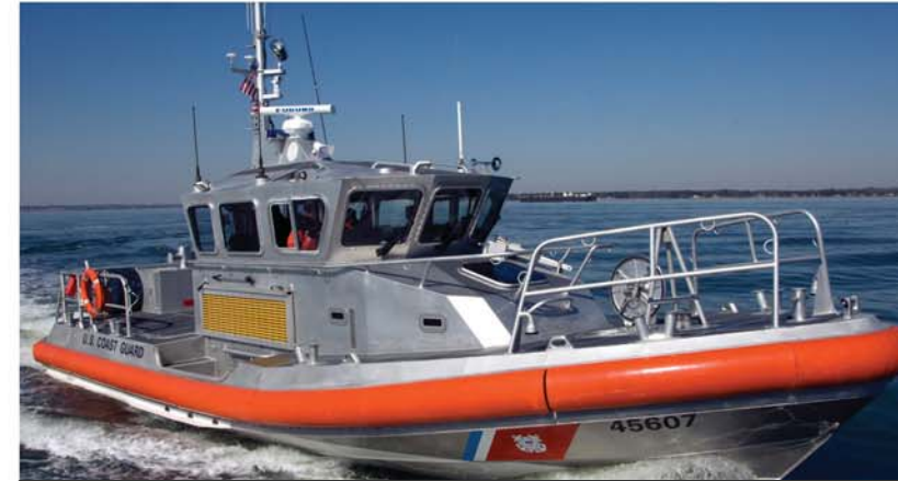
Patrol boat by Kvichak, with Sonihull protection on the hull and twin Rolls Royce water Jets
