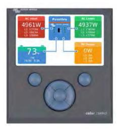
Color Control Panel, showing a PV application
