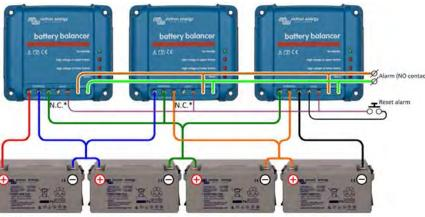
Three Battery Balancers connected to four series
