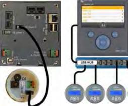
Even more BMVs can be connected to a USB Hub for central monitoring.
