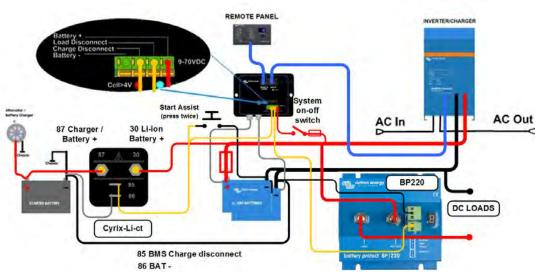
Figure 1: Application example for a vehicle or boat.
