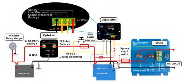
$\label{thm:continuous} \textbf{Figure 2: Application example for a vehicle or boat, without inverter/charger.}$
