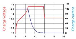
Fig. 3: Three step charge curve
