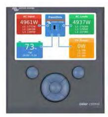
Color Control panel, showing a PV application
