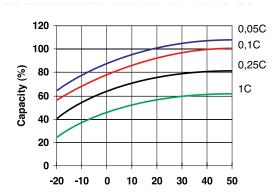
Fig. 1: Effect of temperature on capacity
